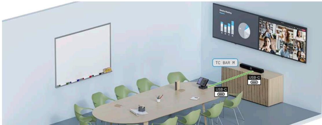
The TC Bar is connected via USB-C® directly to a notebook or or via other UVC- and UAC-capable USB host devices. There is no need for a network connection. In this mode, only restricted functions are available.
